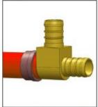
Improperly calibrated tool - not
