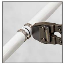
Close clamp ear with ratchet pincer tool. Tool will not release until clamp is fully closed. Remove any defective connections.
