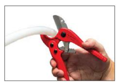
Cut tube at 90-degrees. Do not crush OD of tubing with cutters. Hint: Slightly rotate cutter during blade engagement.
