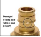
Damaged, cut or grooved barb on fitting.
